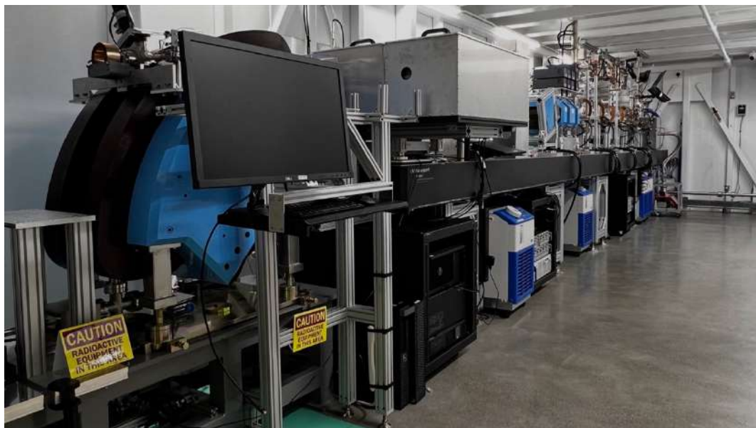
Figure 1: Operational, high-brilliance, distributed charge Compton x-ray source in Irvine, California
